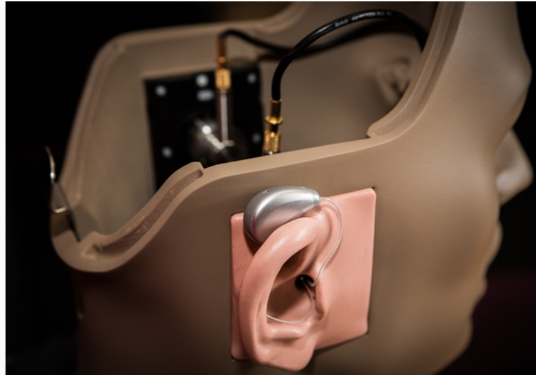
Example setup for open-dome AHA recordings worn by a KEMAR dummy head.
